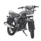
The Company introduced TVS JIVE 110 cc with innovative T-Matic technology in the executive segment which accounts for 60% of the total motorcycle market. This motorcycle allows hands-free gear shift because of absence of the clutch lever. Coupled with this an anti-stall mechanism makes smooth riding possible at low
